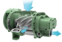
The spiral valve is fully opened, further reducing the effective compression length of the rotor, and the minimum amount of intake air is compressed - the energy consumption is further reduced
